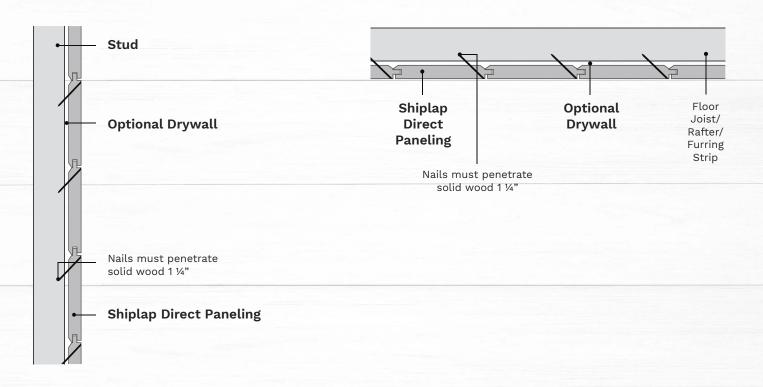
Primed, Raw and Cedar tongue and groove siding can be installed horizontally or vertically. In horizontal application, start at the bottom and work up with the groove edges facing downwards. Siding 6" and 8" wide can be blind nailed through the tongue. Nails must penetrate 1-1/4 inches into solid wood.
