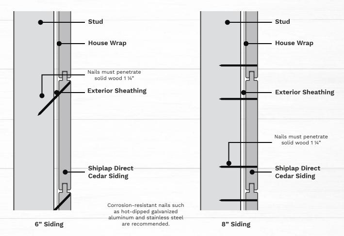
Cedar shiplap can be installed horizontally or vertically. In horizontal application, start at the bottom and work up with the groove edges facing downwards. Siding up to 6 inches wide can be blind nailed with one siding nail per bearing toe-nailed through the base of each tongue. Wider siding should be face nailed using two nails per piece. Nails must penetrate 1 ½" inches into solid wood.
