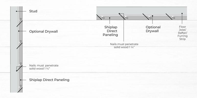
Primed, Fir and Cedar tongue and groove siding can be installed horizontally or vertically. In horizontal application, start at the bottom and work up with the groove edges facing downwards. Siding 6" and 8" wide can be blind nailed through the tongue. Nails must penetrate 1-1/4 inches into solid wood.
